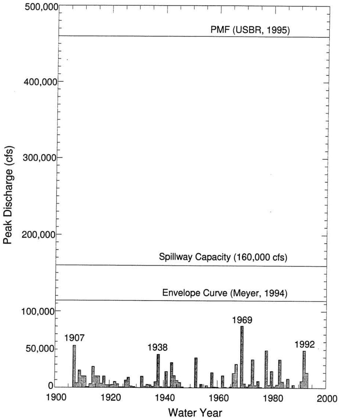
Figure 2. Compiled record of annual peak discharge estimates for the Santa Ynez River at Bradbury damsite. Also shown for comparison are an envelope curve for this part of California from Meyer (1994), the spillway capacity of Bradbury Dam, and the calculated Probable Maximum Flood.
