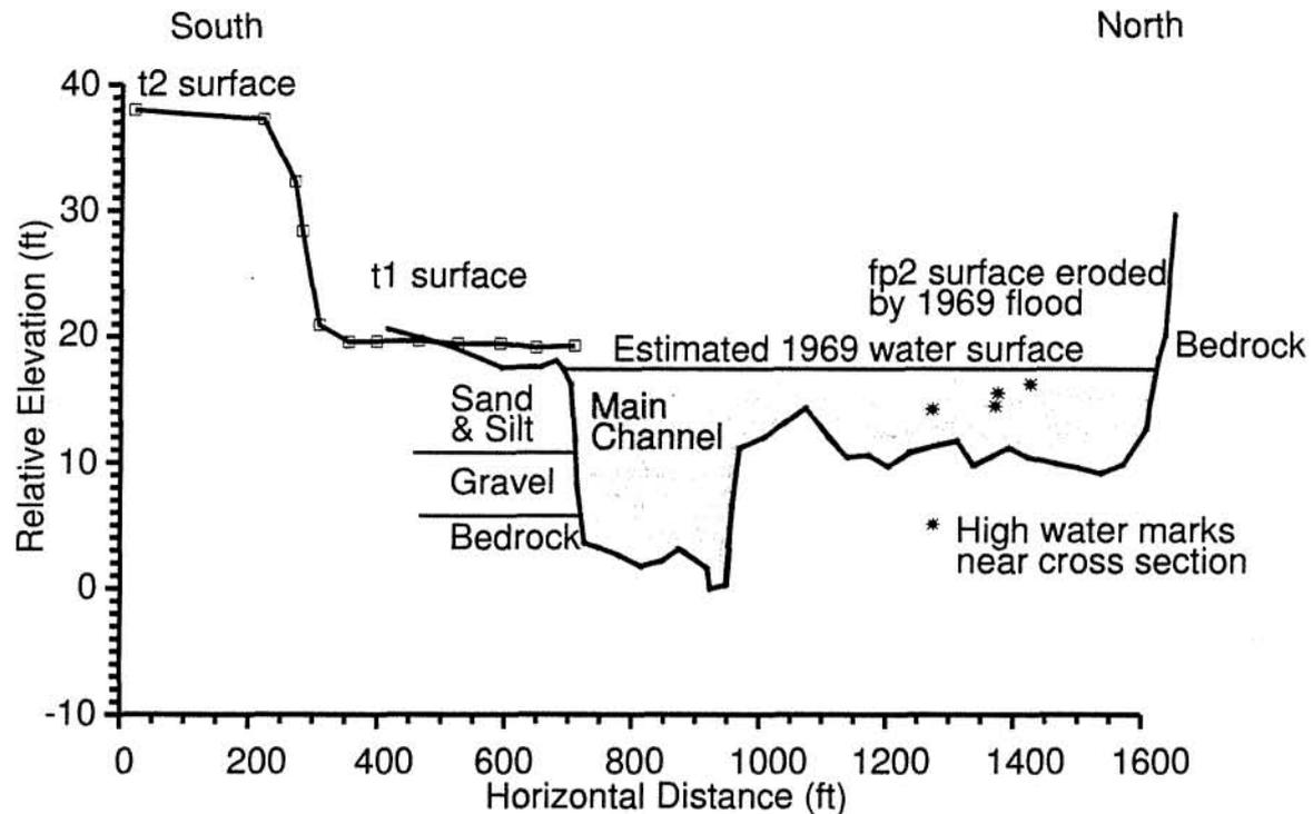
Figure 4. Cross section of the Santa Ynez River at the downstream end of the Crawford study reach. Shallow inundation of the former fp2 surface resulted in severe erosion. The 1969 water surface was up to the margin of t1.
